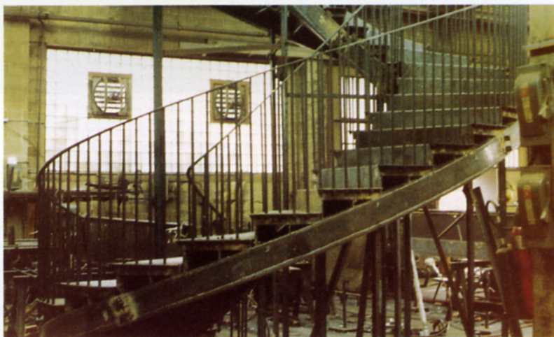
These photos, supplied by Empire City Iron Works, Inc., show the egg-shaped stair as it was fabricated in the firm's Long Island City plant. Below is the finished product. All of the stair's splice plates were welded up and ground smooth before the final wood finish was added.
